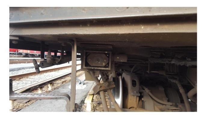
Figure 5. Red Line Emergency Bypass Switch (Outside View)
